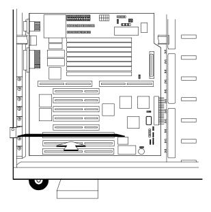
Figure 3-7. Installing a Board
